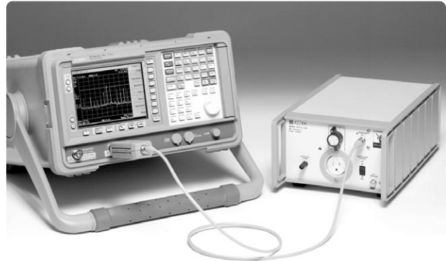
Use the EMC analyzer with the 84115EM-11967D LISN device to test for conducted emissions.
